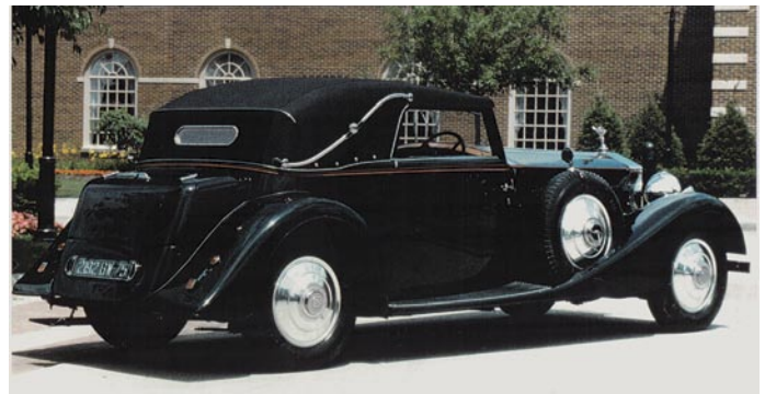
From its previous restoration, the most notable changes—guided by the Bulletin photos—are the fender sidelamps and tail lamps, the spotlamp, the license plate configuration and holders, the coloring of the wheel discs, and the addition of a cover for the spare wheels.
